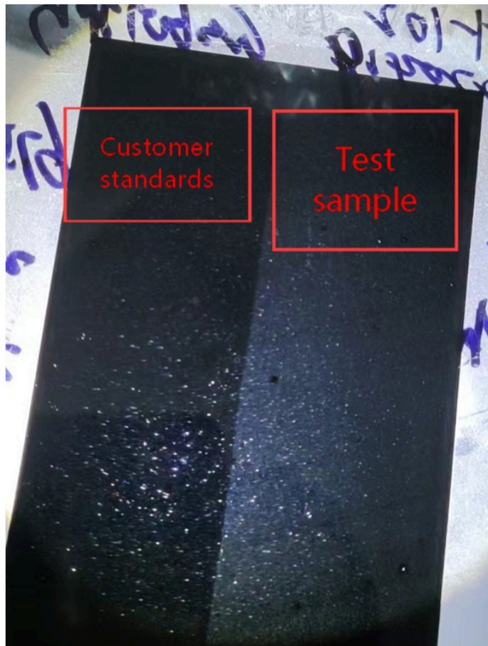
Issue: poor covering(hiding) power
